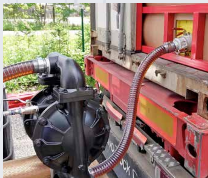
High fluid viscosity reduces pump delivery.
